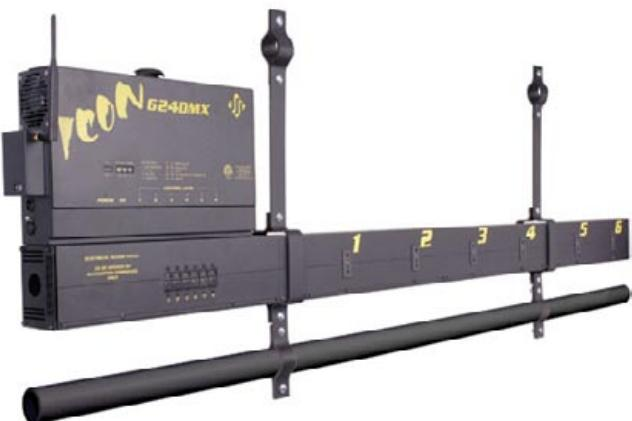
Johnson Systems engineering team drew on their experience with retrofit installations to design the ICON Series of dimmers that are simple to install, operate and service. All ICON Series dimming products feature industry-standard 2.4kW dimmers built to unparalleled standards and use readily available "non-proprietary" parts to maximize product lifespan and permit ease of future serviceability.
